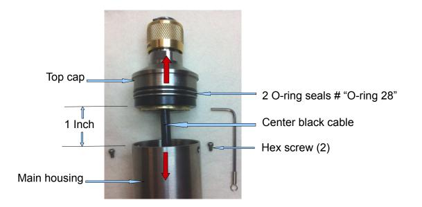
3- The 8 batteries are inside the main housing in four separate compartments. Install new batteries following the polarity as indicated by the battery label.
