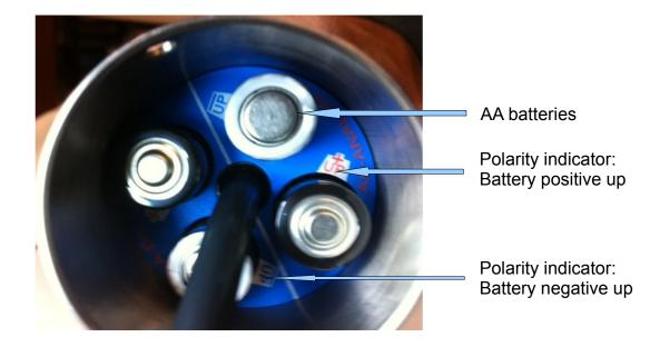
4- Before closing the unit, make sure the o-ring seals are not damaged. Replace if needed with part number "O-ring 28."
