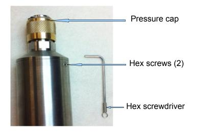
2- Pull the top cap and the main housing apart for about 1 inch (2.5 cm). The black cable at the center is attached to the connector cap and should pull smoothly through the center of the battery housing.
