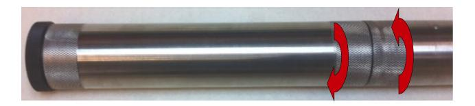
3- Remove the "Storage / calibration cup" from the sensor guard and deploy the unit.
